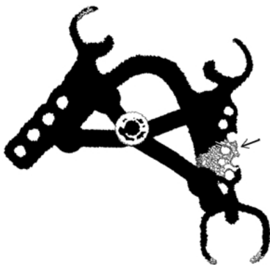
Figure 5 Filling result of the lower jaw framework with ball sprue. 95% filled at time 0.191 s.
