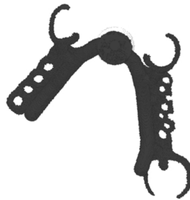
Figure 6 Filling result of lower jaw framework with runner bar sprue. 95% filled at time 0.245 s.
