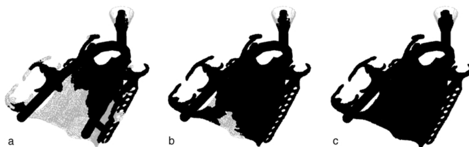
Figure 8 Filling sequence of the upper jaw framework with runner bar sprue. (a) 80% filled at 0.248 s, (b) 90% filled at 0.339 s, (c) 95% filled at 0.375 s.
